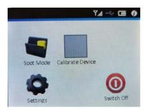
The "Calibrate device" button performs an automatic calibration of the device by automatically inserting the internal reference white and performing calibration.
