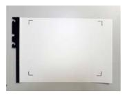
This sample holder is made of a selected white material conforming to ISO 13655-2017.
