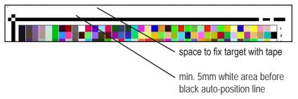
If the sensing unit is connected to the platform, the autopositioning is done by taking a picture with the camera and calculating the corner points by the sensing unit.
