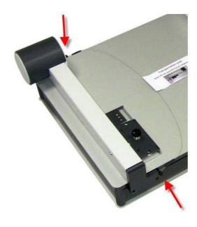
4. The next step is to add the protective foam under the measurement head, to fix it with the rubber band and to give the LFP into the nylon bag:
